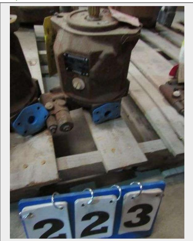
REXROTH/DAN FOSS, AXIAL HYDRAULIC PUMP #R902502726/000A10V028DFR/31R-VSC62N00, 28 CC, 22 GPM, CAMERON #2360642-05, CO. #19-8, INTERNAL PORTS INSPECTED AND ARE RUST FREE INSIDE, EXTERIOR RUST ONLY
